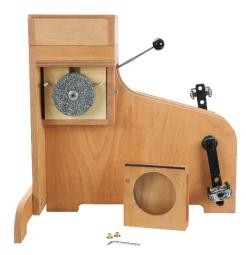
Nevertheless, if the grinding stones are smeared, it is advisable to grind some rice on a medium-coarse setting. The rice removes the fats and moisture from the stone that caused them to stick together.
