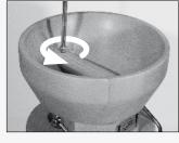
You can now lift out the hopper. Ensure that you retain the foam rubber ring. This is either loose or attached to the hopper. Replace it when reassembling the machine.
