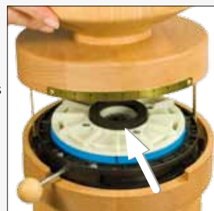
Figure 9 Make sure the foam rubber gasket is properly seated (arrow). Return the funnel to its previous position and secure it with the brass screws.
