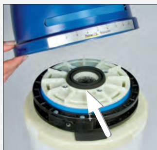
Figure 9 Make sure that the foam rubber gasket is properly seated (arrow). Mount the funnel and secure with the funnel bracket screw and adjusting lever.
